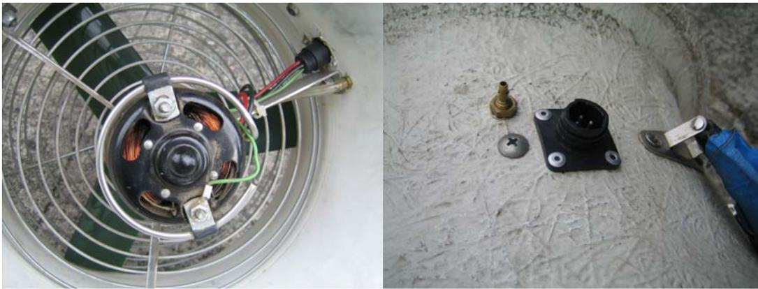
The amount of air going through the fan assembly is controlled by a rheostat operated by the tester. Depending on the amount of air that is being measured, a black plastic flow restriction ring may be needed. The flow restriction rings are also round, smooth orifices that increase the pressure drop across the entire fan assembly, thereby increasing the accuracy of the measurement. When the pressure drop across the fan assembly drops to below about 20 Pa, it is time to
