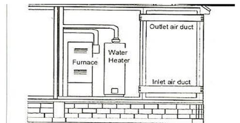
the following applies: When using a single opening it must have a free area of one sq. in. per 3000 BTU's of total input rating for all appliances. When considering the location of outside air louvers make sure nothing is being vented near enough to allow that unit's products of combustion or possible corrosive when burned fumes to be draw into your openings.
