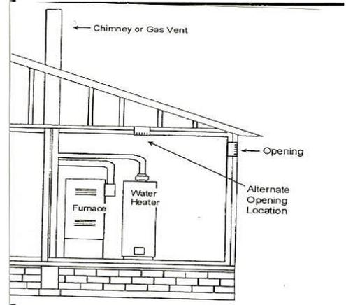
Recirculation of vented combustion products can cause combustion issues due to their lack of oxygen.
