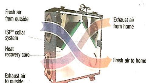
central heat-exchanger core that extracts the heat from one air stream and transfers it to the other but does not mix the air streams together. In most units the incoming air is filtered on its way through.
